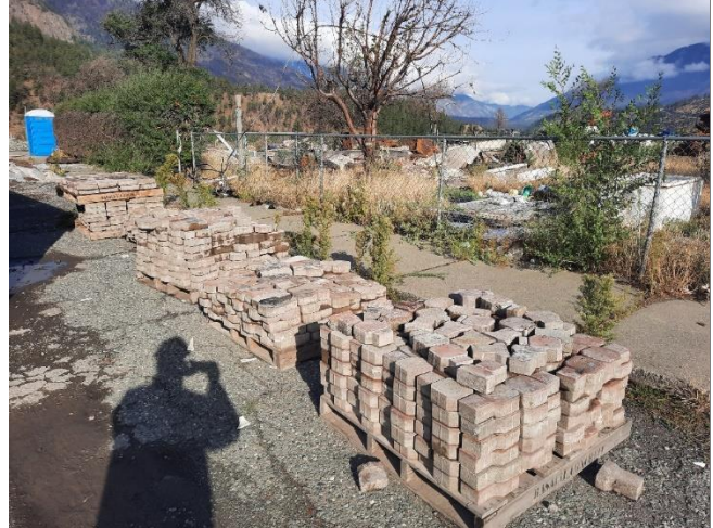
Figure 8 – Salvage bricks for re-use
